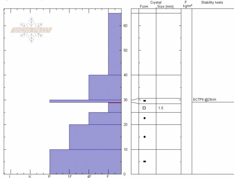
Notes: After the first ectp on the ice/faceted interface on a 17 degree slope we dug two more ect s within 50m area on approximately North facing as degree slope with propagation upon block seperation, the other on a 10 degree slope with ectn 11 on the same layer.
