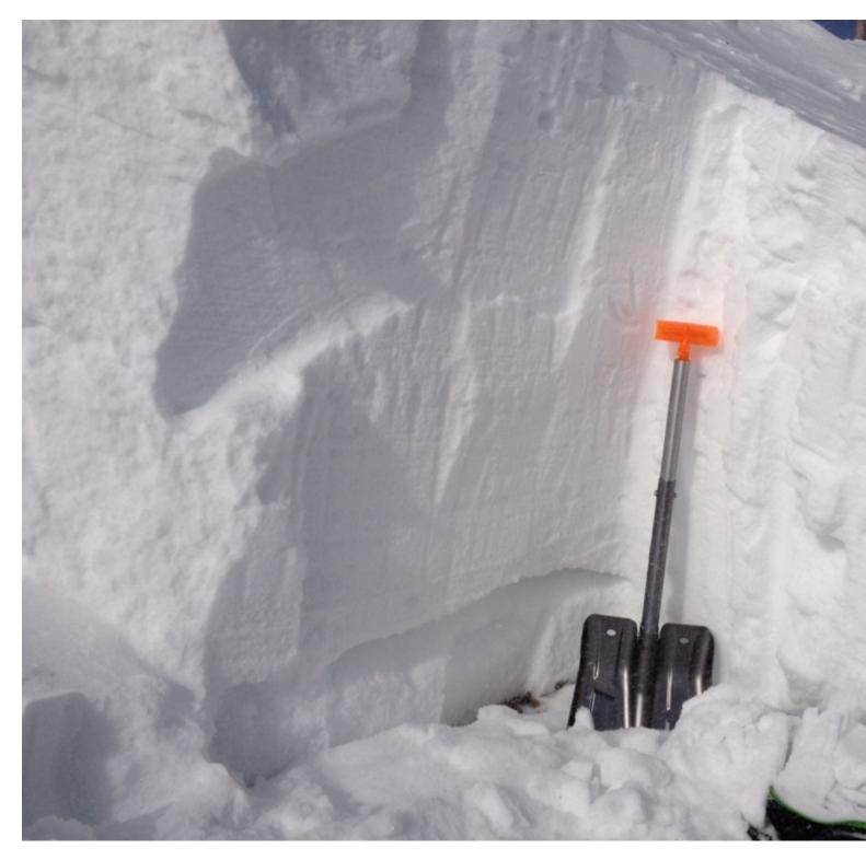
This is the crown of the Football Field avalanche on Saddle Peak. (P+ slab; 3 ft to 7ft deep; 2-4mm fx F hardness). It broke on weak facets about a foot above the ground. Photo: GNFAC
