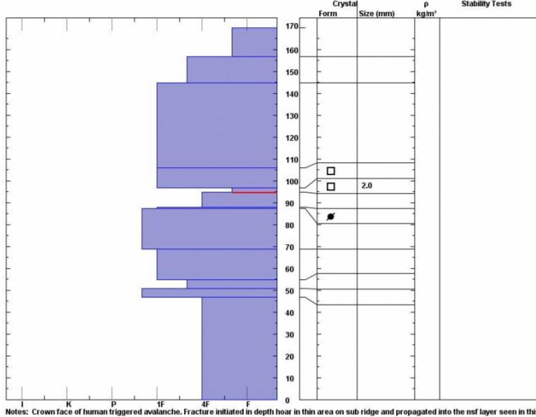
Notes: Crown face of human triggered avalanche. Fracture initiated in depth hoar in thin area on sub ridge and propagated into the nsf layer seen in thi Average starting zone angle 36 degrees.
