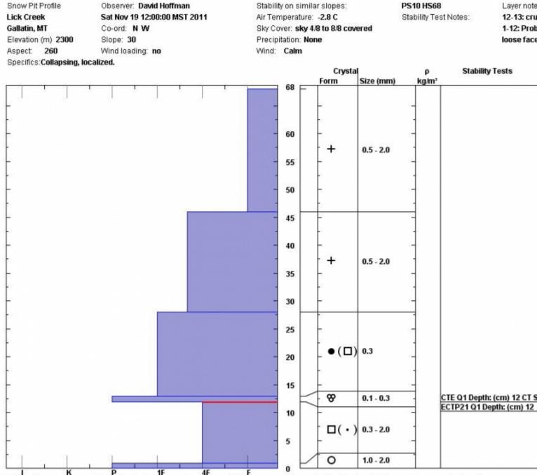
I K P 1F 4F F U Notes: There is a layer of loose faceted grains under a thin crust that appears to be unstable. The faceted layer collapsed while traveling on a nearby s ECT score may have been deceptively high due to the depth of the layer.
