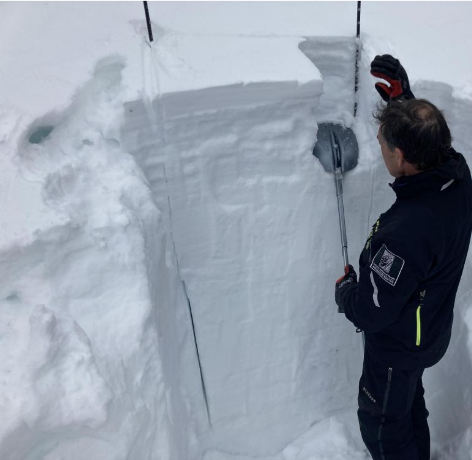
Doug Chabot performing an ECT in a 6 foot deep, generally stable snowpack near Tincup Pass in the Centennial Mountains (outside Island Park). 3/2/22. Photo: GNFAC
