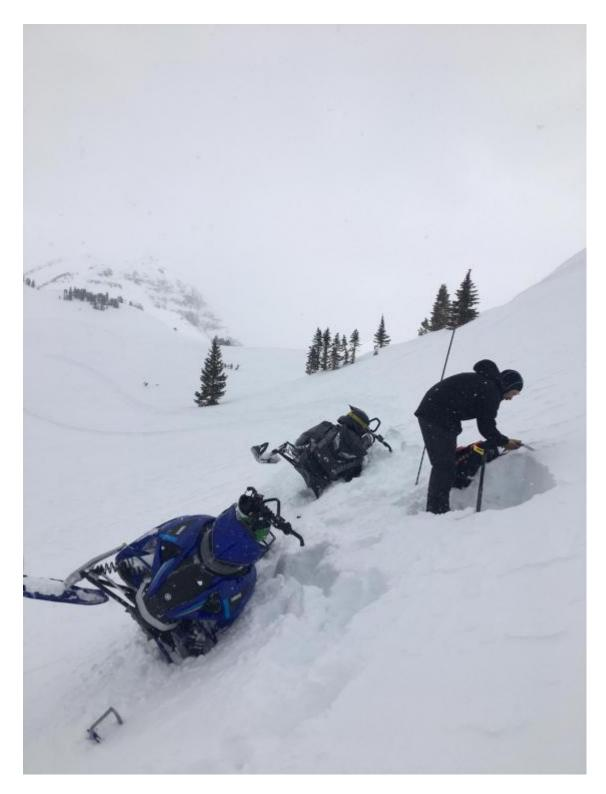
Ian and Dave stop to do a quick stability test as they hunt for a layer of weak snow 1-2 feet under the surface. Photo: GNFAC
